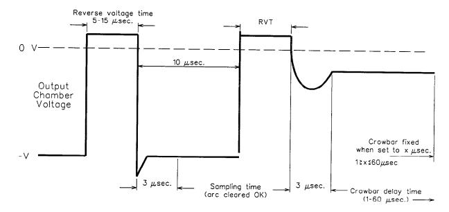
Figure 3-2. Crow-bar Delay Time example
