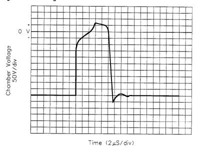
Figure 2-1. Chamber voltage during Passive mode.
