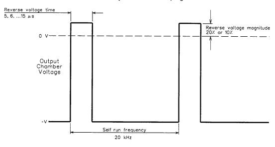
Figure 3-1. Reverse Voltage Time (RVT) example
