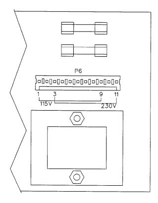
Figure 2-6. Changing the AC Line Voltage (115 V or 230 V)
