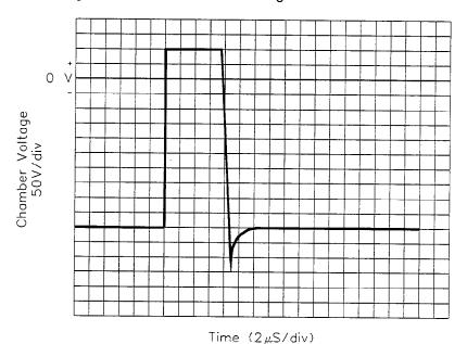
Figure 2-5. Chamber voltage during Self-run mode.
