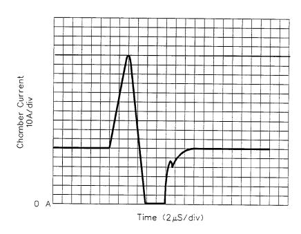
Figure 2-2. Chamber current during Passive mode.
