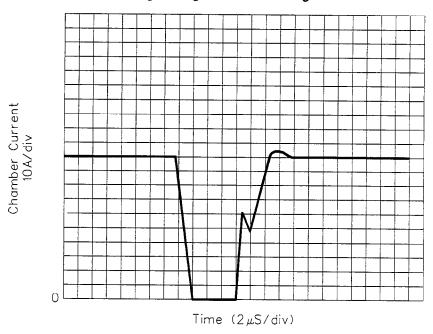
Figure 2-4. Target current during active arc-handling mode.
