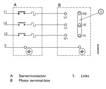
Figure 6 – Three-phase electrical connections: 380-460 V
