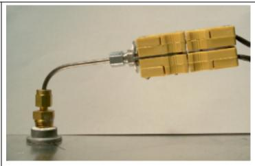
Figure 1-32 Dual Thermocouple Installed
