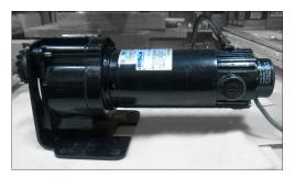
Figure 1-22 Drive Motor, Medium Speed
