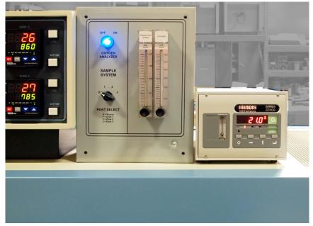
Figure 1-37 Oxygen analyzer next to OSS sample system
