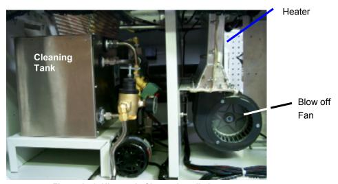
Figure 1-46 Ultrasonic Cleaner installation
