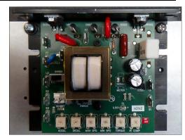
Figure 1-20 Motor Controller
