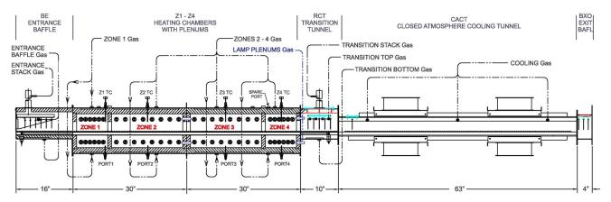
Figure 1-9 4-Zone CU-900 Series Internals
