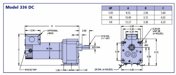
Figure 1-23 DC Drive Motor, Medium Speed
