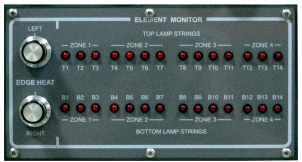
Figure 1-33 Zone Lamp Element Monitor Panel
