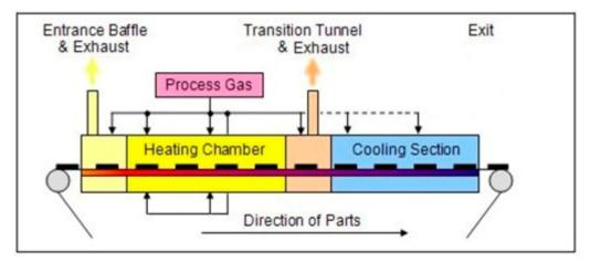
Figure 1-8 Process Sections
