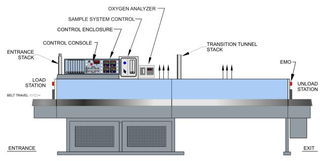
Figure 1-1 CU-915 IR Furnace Front Elevation
