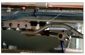
Figure 1-44 Sample Port Chamber Penetration
