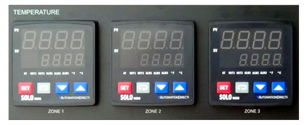
Figure 1-18 Zone Temperature Controllers
