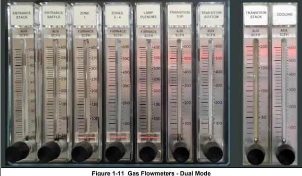
Each flowmeter is identified with a label as to specific function and is adjustable from zero flow to full scale by means of a needle valve control knob. Turning this knob CW decreases flow; CCW increases flow. Flow is read on the graduated scale at the mid-point of the bead.
