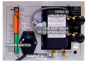
Figure 1-39 EC913 Oxygen Analyzer Rear Controls
