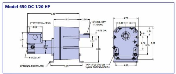
Figure 1-25 DC Drive Motor, Low Speed
