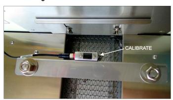
Figure 1-43 Calibrate Sensor
