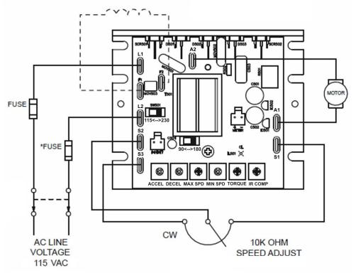
Figure 1-21 PCM23011C Motor Controller
