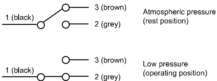
Fig. 2 Contact assignment of microswitch
