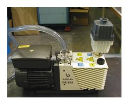
Mist Eliminator mounted on top of Vacuum Pump. (Oil pumps)
