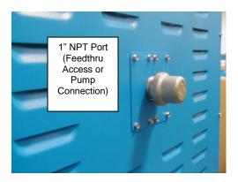
Locate the fittings at the rear of the oven as pictured. Locate the  $\frac{1}{4}$ " and  $\frac{3}{8}$ " diameter Vacuum tube(s) packaged inside the oven. These tubes are barbed at the end for easy connection.
