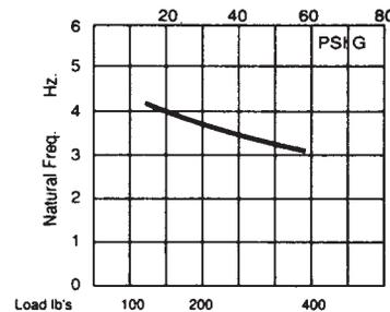
Note that even though the natural frequency of the isolator is reduced when the load increases, there is little change in the transmissibility curve and the resulting isolation capability. In fact, the load is a function of the microscope or equipment weight and, thus, is not variable in any given application. NTA's Isolation Units will isolate close to 90% of input vibration amplitude within the 20-75 HZ frequency range, in all three axes.
