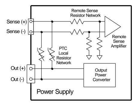
Figure 3-22. Remote Voltage Sensing Network
