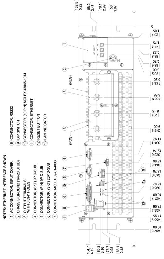
Figure 2-10. Rear Panel, Ethernet Option, 3U Models 10V-30V
