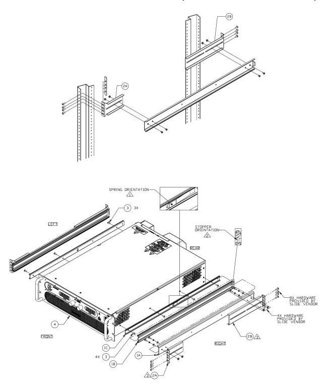
Figure 2-1. Rack Mount Assembly for 3U Models
