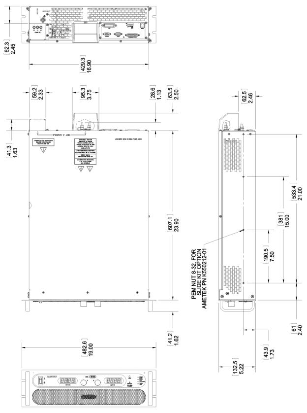
Figure 2-6. Installation Drawing, 3U Models 800V-1000V
