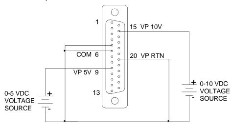
Figure 3-16. Remote Voltage Programming Using 0-5 VDC or 0-10 VDC Source
