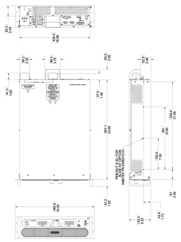
Figure 2-5. Installation Drawing, 3U Models 40V-600V
