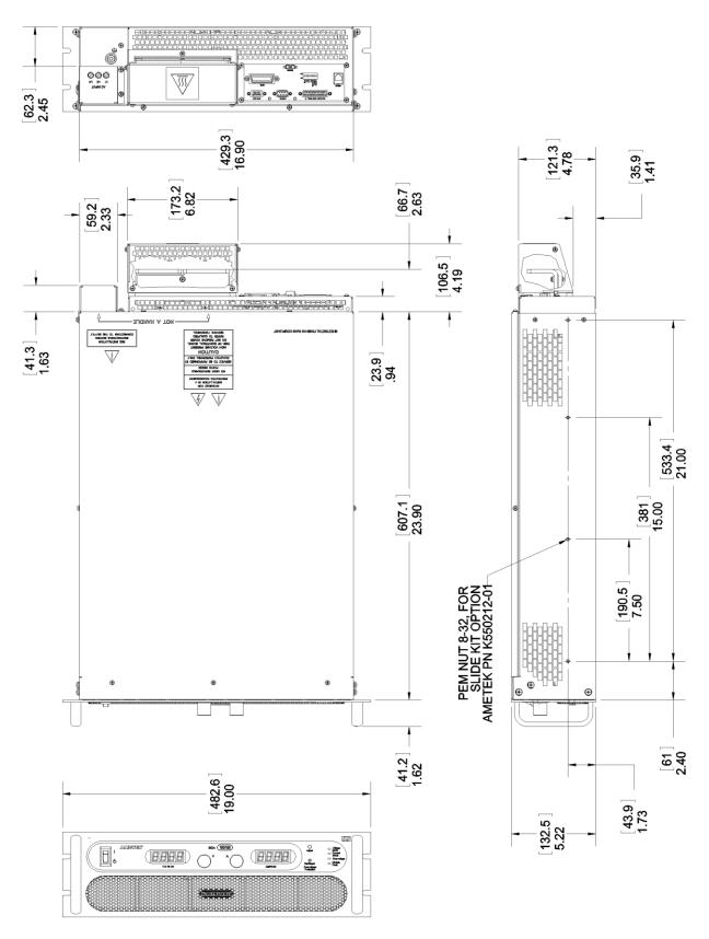
Figure 2-4. Installation Drawing, 3U Models 10V-30V
