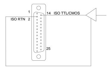
Figure 3-20. Remote Output ON/OFF Using Isolated TTL/CMOS Source
