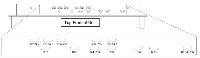
Top view of potentiometers as located on internal circuit boards.
