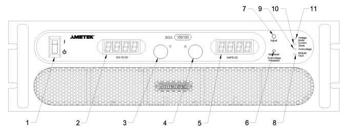
Figure 3-1. Front Panel Controls and Indicators (3U Model Shown)
