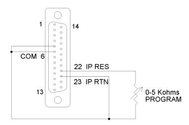
Figure 3-13. Remote Current Programming Using Resistance
