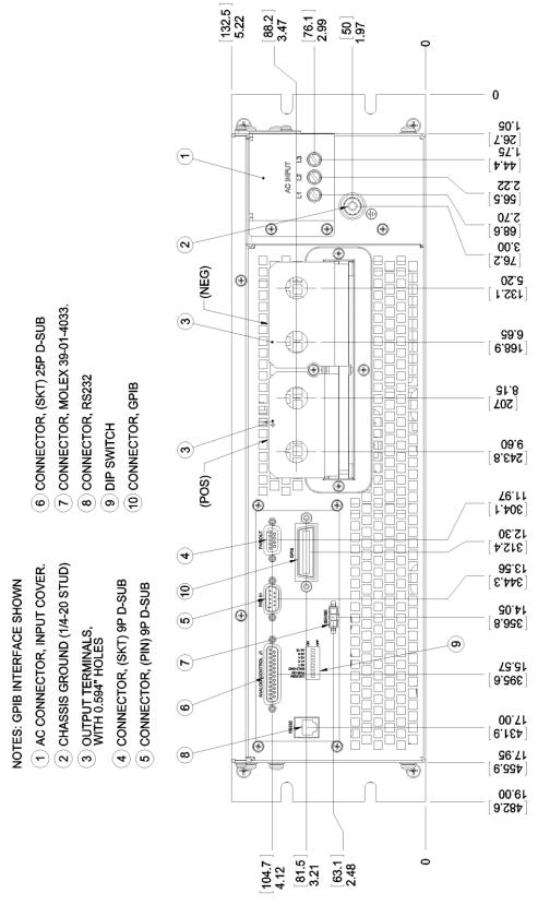
Figure 2-9. Rear Panel, GPIB Option, 3U Models 10V-30V
