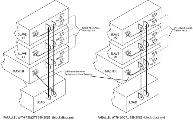
NOTE: The voltage display on the slave units will be slightly higher than the master unit. The twisted pair cable length must be as short as possible.
