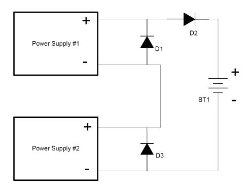
Figure 3-26. Series Connection with Anti-Parallel Diodes
