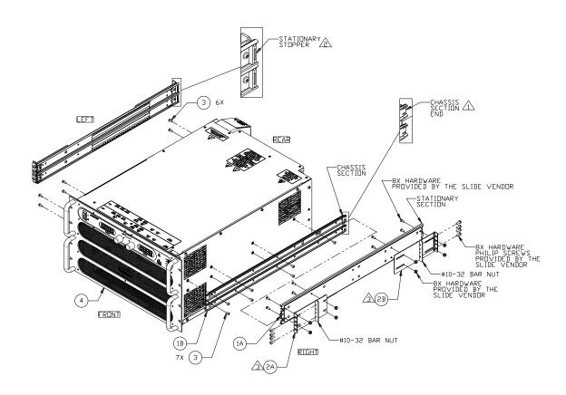
Figure 2-2. Rack Mount Assembly for 6U Models
