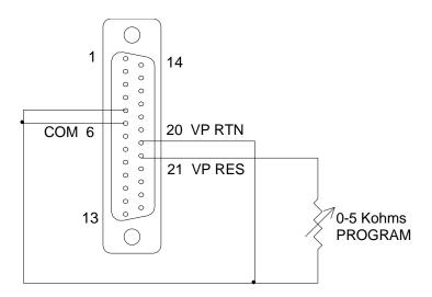
Figure 3-15. Remote Voltage Programming Using Resistance
