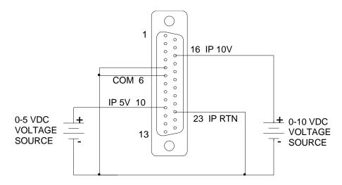
Figure 3-14. Remote Current Programming Using 0-5 VDC or 0-10 VDC Source
