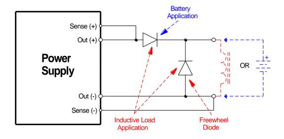
Figure 2-3. Diode Connection
