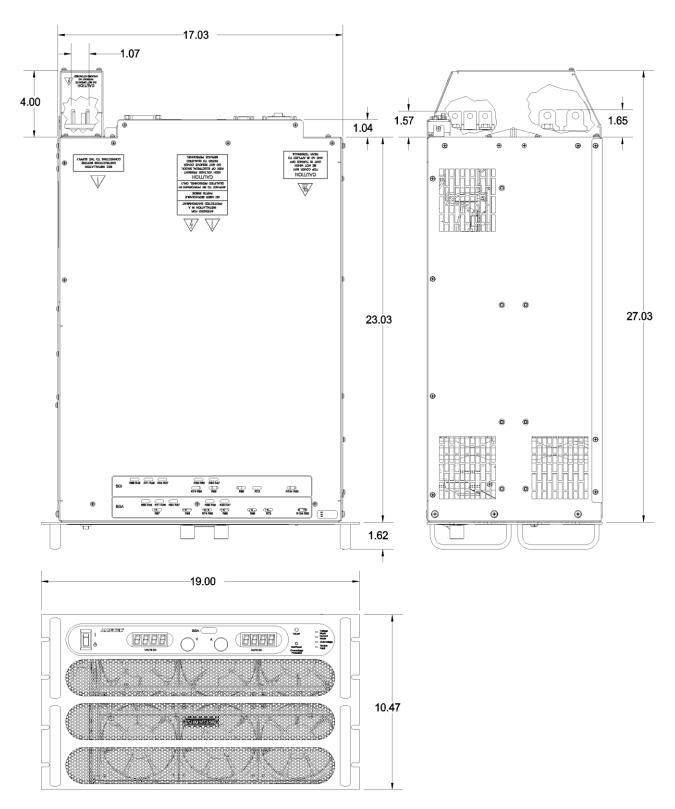
Figure 2-7. Installation Drawing, 6U Models 20 kW to 30 kW
