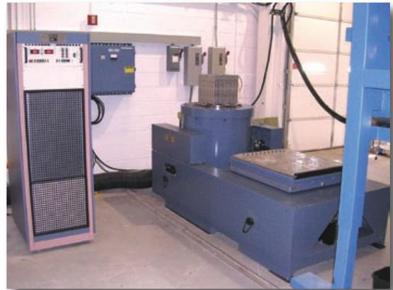
H560B-16 with Slip Table Assembly and a Cube Fixture
